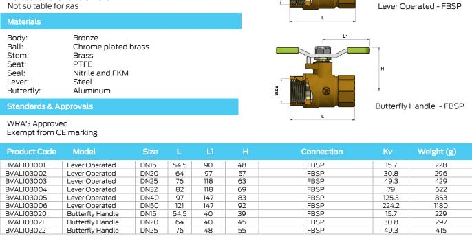
All dimensions in mm unless otherwise stated Kv is the headloss across the complete valve in the fully open position
