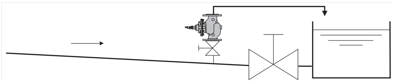
Fig. 1 Standard installation example for the safety valve
